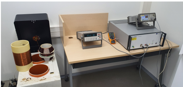
Fig. 2: Proposed and constructed experimental setup showing the applicator used in preliminary experiments and the newly designed applicator.
